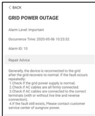
figure 7-9 Detailed Fault Alarm Information
